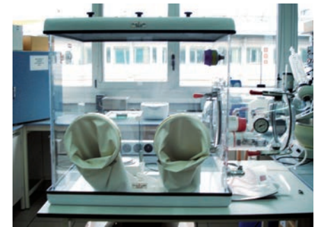
Glove box for reactive compounds handling
