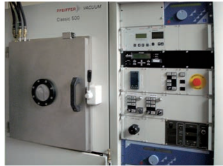
Sputtering machine for thin film deposition
