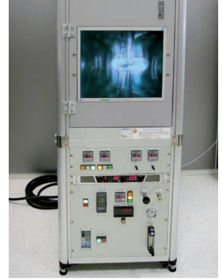
Floating zone furnace for single crystal growth
