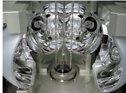
Detail of the ellipsoidal mirrors of the floating zone furnace for single crystal growth
