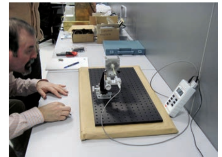
BCMaterials researchers testing a focusing magnetic quadrupole for proton accelerators
