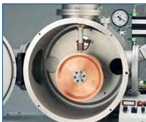
Detail of the vacuum chamber, crucible and spinning wheel
