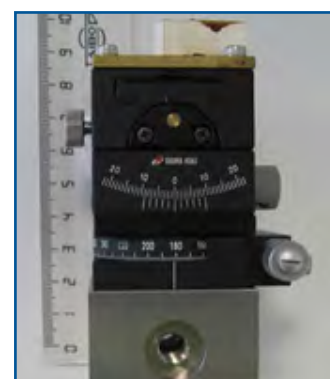
Scheme of the new LAUE diffractometer (Left). View of the goniometer (Right)
