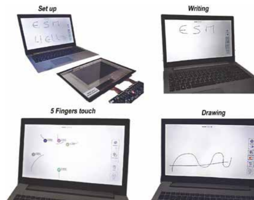
Fig 2 Illustration of the device based on a screen-printed flexible matrix using water-based graphene nanoparticles inks with cellulose as polymer binder.
