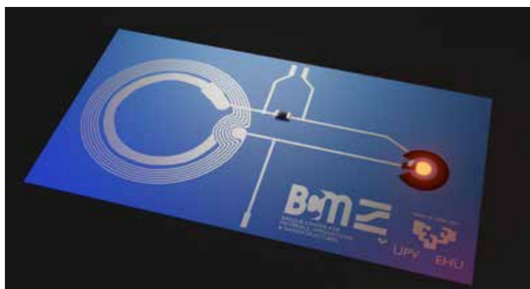
Fig 1 A photorealistic render of the NFC electrochemical platform for electrogenerated chemiluminescence point of care devices.
